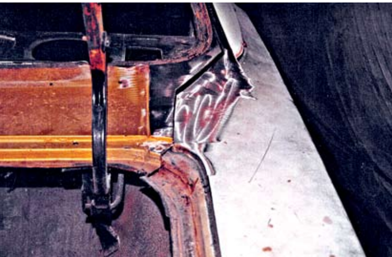
This is the right side of trunk drain; the tin worm had rotted out this piece; Watson, again, precisely cut, carefully welded and made metal fit like new
