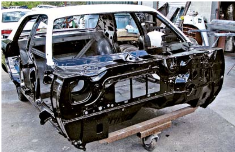
Here is finished body minus the fenders and radiator support awaiting assembly on a home-made dolly; attention was given to prepping firewall
