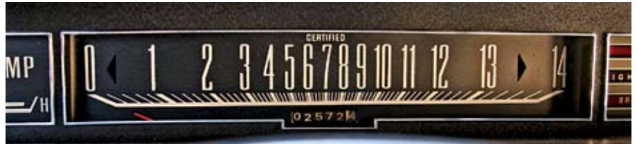
Note “Certified” bar speedometer to 140 mph and period-correct Federal Interceptor police radio
