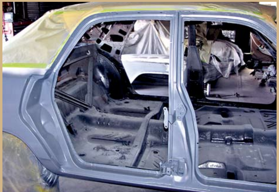
Here the body is primed; roof is taped off to avoid overspray; the white paint has been applied and the painter has prepared the door jambs and quarter panels for the black paint to be applied
