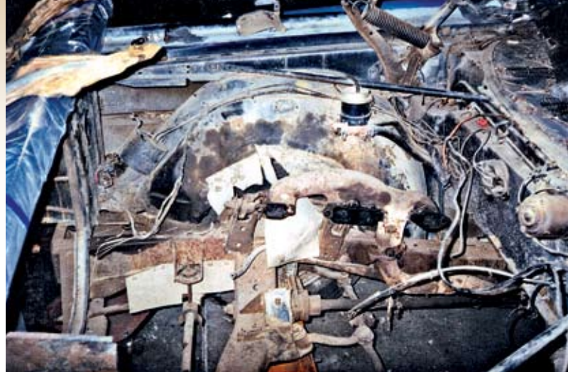
Many hours were spent removing all the parts from the crusty engine bay; car's entire front end was rebuilt; the firewall was stripped and refinished
