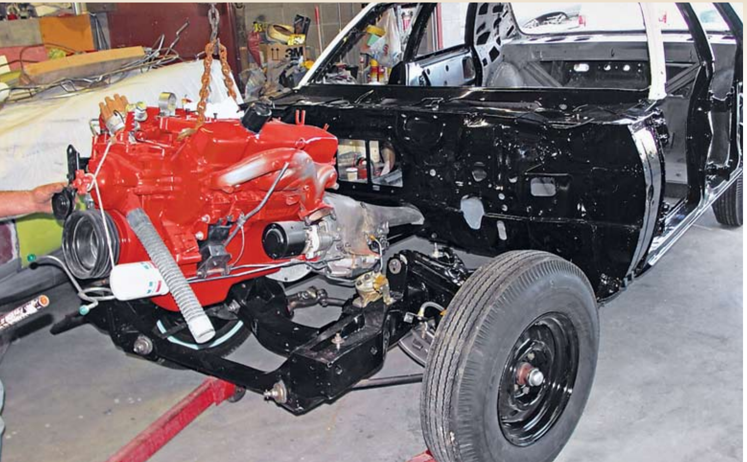
Milestone: the rebuilt and detailed engine being lowered into the restored frame; the remaining sheetmetal was then bolted to the car and aligned to fit
