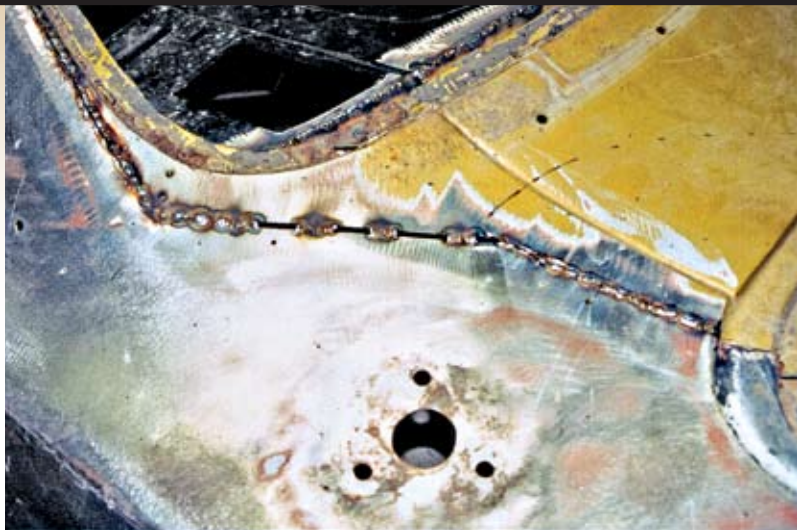
From the top of the rear window to the trunk drain, Watson performed very tricky surgery; he tack-welded the metal into position then ground it to fit
